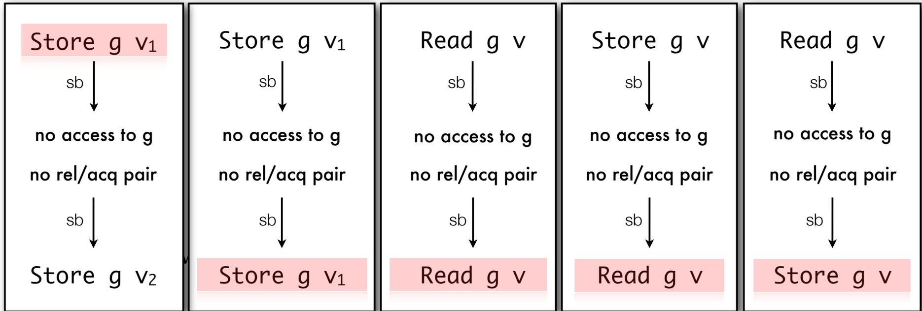
Overwritten-Write Write-after-Write Read-after-Read Read-after-Write Write-after-Read
