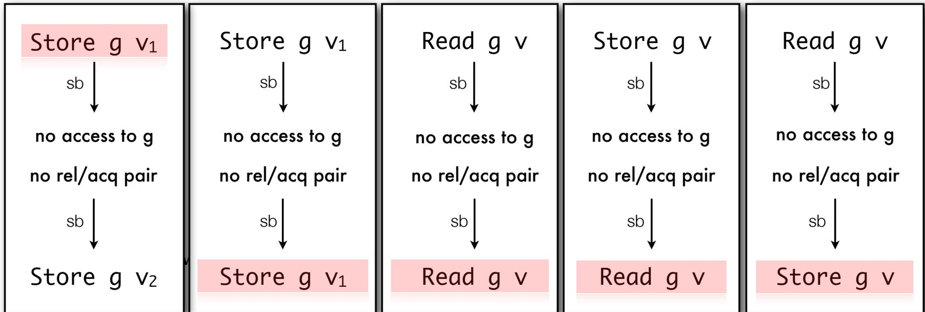
Overwritten-Write Write-after-Write Read-after-Read Read-after-Write Write-after-Read
