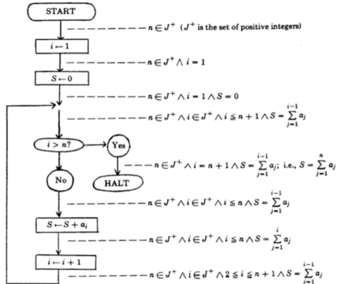
FIGURE 1. Flowchart of program to compute  $S = \sum_{j=1}^{n-1} a_j$  ( $n \geq 0$ )
